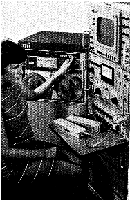
The "Autotest" response measuring system incorporating Siemens programmable instrumentation in use at the St. Albans factory of Marconi Instruments to check out filters from the large scale production of White Noise Test Sets.
